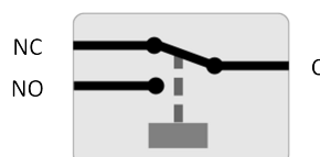
Relay configuration (not energised).
