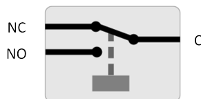
Relay configuration (not energised).
